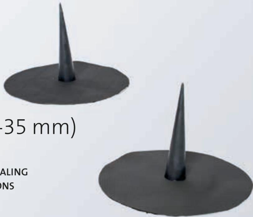
EPDM shaped part for slipping over and sealing in roof penetrations with a round cross-section and diameters of 5 to 35 mm. The connecting collar consists of a circular piece of RESITRIX® SK W Full Bond with a diameter of up to 30 cm.
