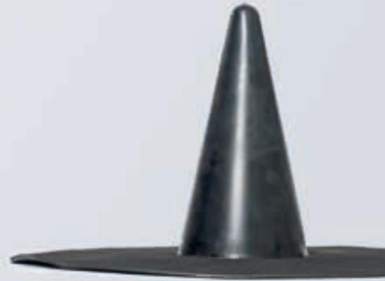
EPDM shaped part for slipping over and sealing in roof penetrations with a round cross-section and diameters of 35 to 100 mm. The connecting collar consists of a circular piece of RESITRIX® SK W Full Bond with a diameter of 50 cm.
