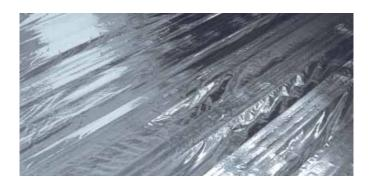
Vapour barrier consists of bitumen membrane covered with aluminium foil. This membrane is intended for application on the metal profiled decking as the vapour barrier layer of the roofing system. Suitable for application in roofing systems of civil and industrial buildings with normal and increased temperature and moisture regime (factories, gyms, pools).
