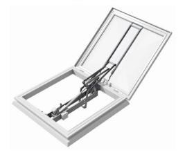
Providing excellent insulation, triple skin Mardome rooflights achieve a centre pane U-value of 1.8  $W/m^2K$  with a  $U_d$ -value which ranges from 1.37  $W/m^2K$  to 1.49  $W/m^2K$  depending on size.
